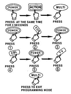
Pressing the (MULT) button will now activate the VCR Power/On, Cable Box Power/On, and the Receiver Power/On at the same time.
